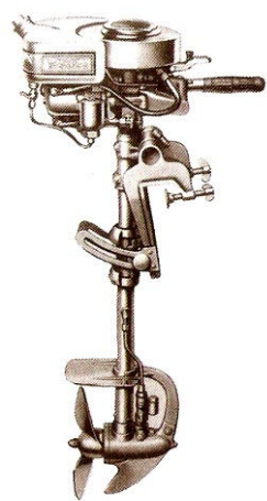
Johnson Water Bug, Model J-25, 1.5 hp motor, 1925-32, The Old Outboard Book
